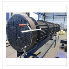
Copper Heat Exchanger Retubing
